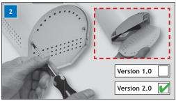
Remove the two screws and remove the metal plate in the bottom of the fog cannon. Remove empty fluid bag if any.
