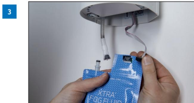
Remove the fluid hose from the empty bag by pressing the metal part at the end of the hose. Also, remove the cord by pressing the bottom of the plug, and then carefully pull it out.
