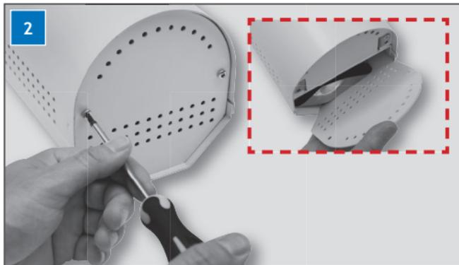
Remove the two screws and remove the metal plate in the bottom of the Fog Cannon™. Remove the empty fluid bag.
