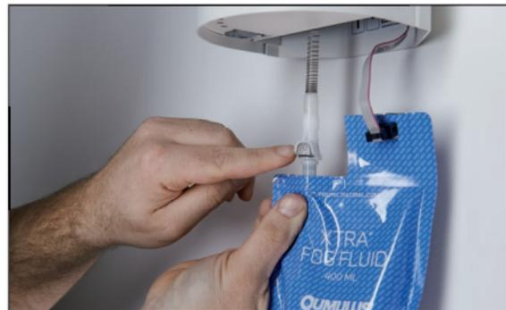
Connect the fluid hose and cord to the new bag and push it up into the machine. The hose coupling must click and the little metal part jump out. The metal plate is screwed back on.
