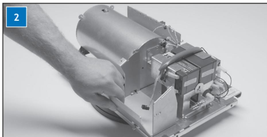
Place the supplied metal plate as shown in the diagram and push it a little to the left until it clicks into place. Attach the metal plate to the base plate with a screw (T20).
