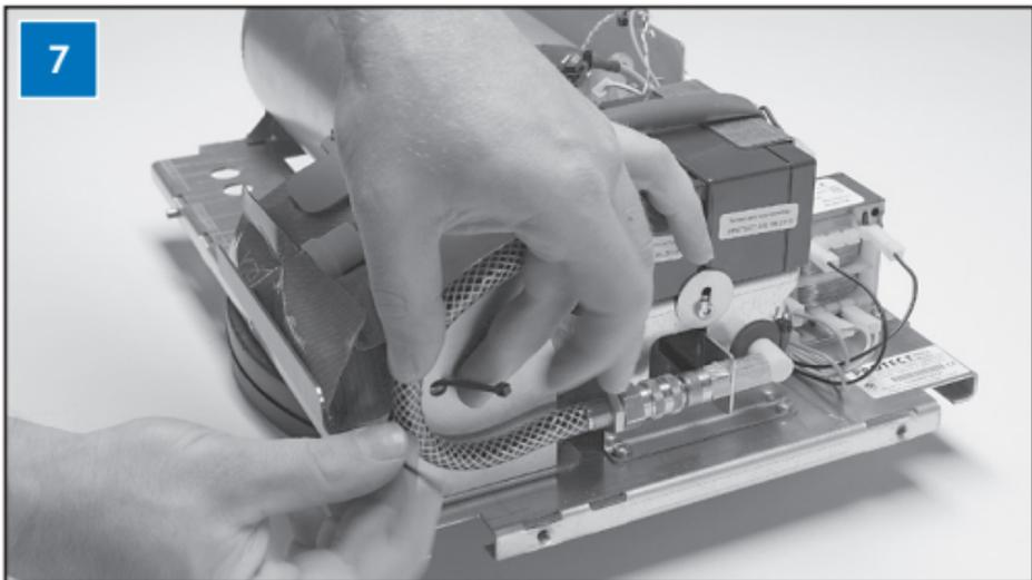
Now the strip can finally be tightened around the fluid hose. **IMPORTANT:** Do not tighten too tight or too loose!
