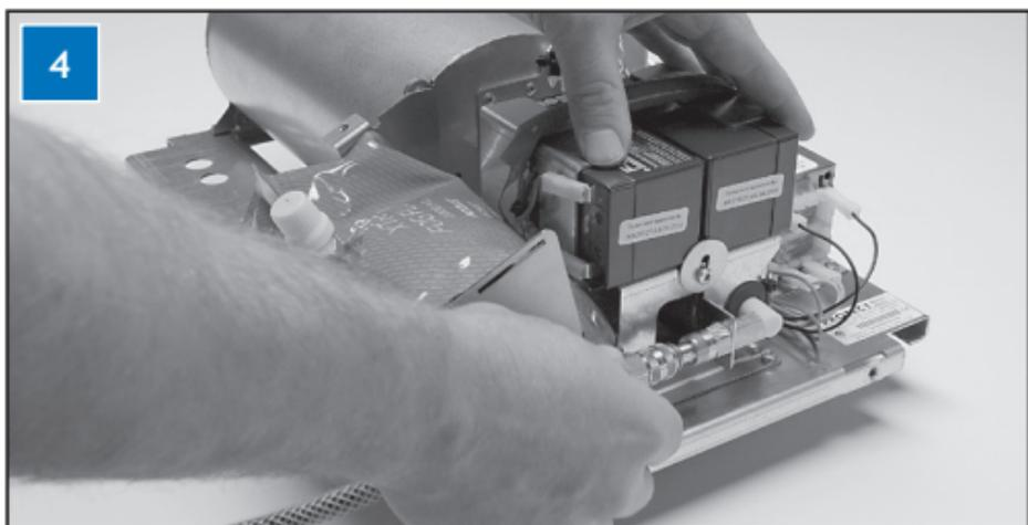
Connect the fluid hose to the unit. When you hear a “click” it is properly in place.
