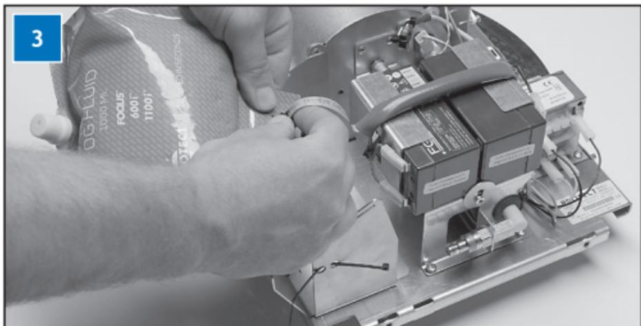
Connect the fluid bag to the cord and place it in the holder. Now thread the heat resistant strip through the two holes in the metal plate (but do not tighten the hose with the strip just yet).
