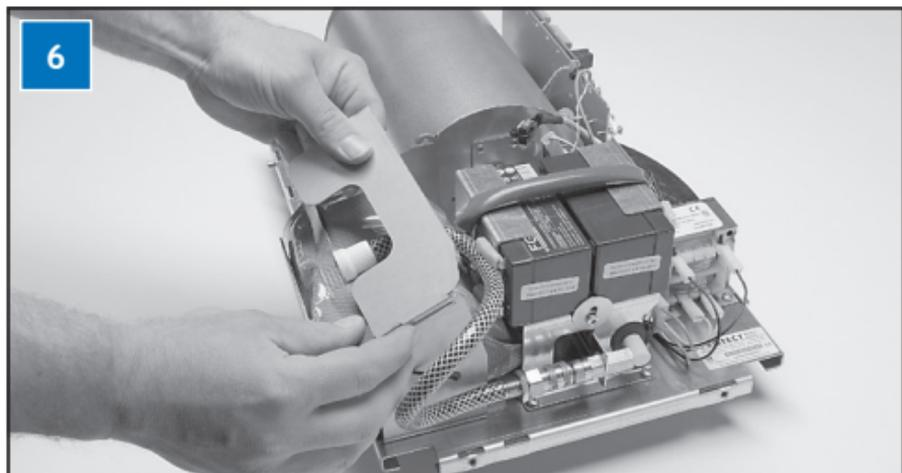
Place the top cover in the corner to the right and screw it on the opposite side with the supplied screw. **IMPORTANT:** The top cover must not trap the fluid bag's cap and ensure the hose is placed between the two poles on the battery.
