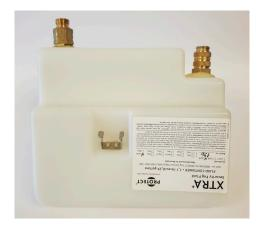
The images below represent a container in good condition. The container should appear clean, similar in colour to the images below and without cracks or deviations. Brass fittings should be fully intact, have a bright finish and undamaged.
