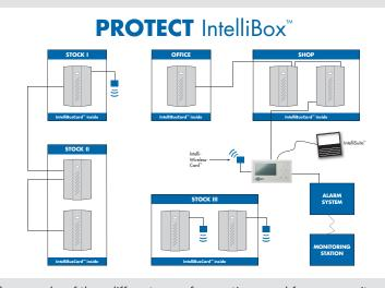
Each IntelliBox can control up to 16 fog cannon units. Depending on the security class required, you either choose a wireless connection (A) or a cabled connection (B) - or a combination.
